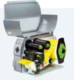
On request, the A4<sup>+</sup> and A6<sup>+</sup> transfer printers are also available with a metal cover. (as standard for the A8<sup>+</sup>).
